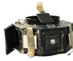
Multiple pinhole panorama camera Film: 120 roll
